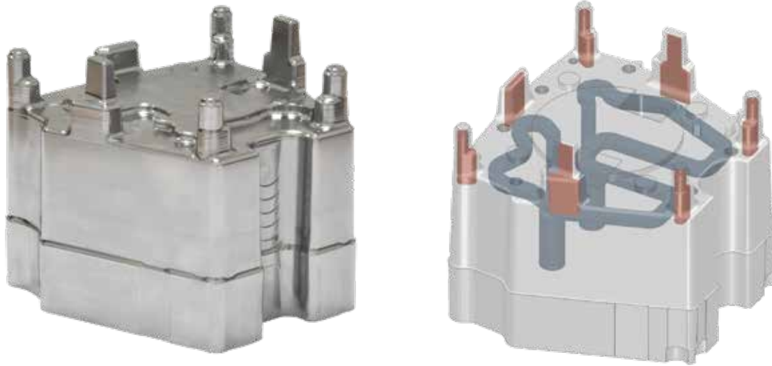
Injection mould with optimised cooling. Copper elements in the extremities which are not accessible to a channel dissipate the heat to the lower cooling channel.
