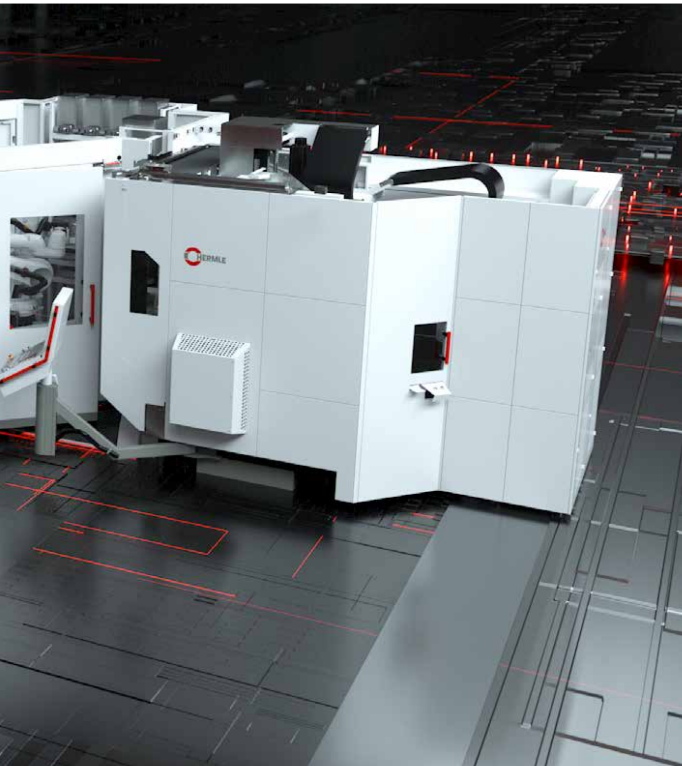
The RS-1 robot system adapted to two 5-axis machining centres C 22 U of the High-Performance-Line series.
