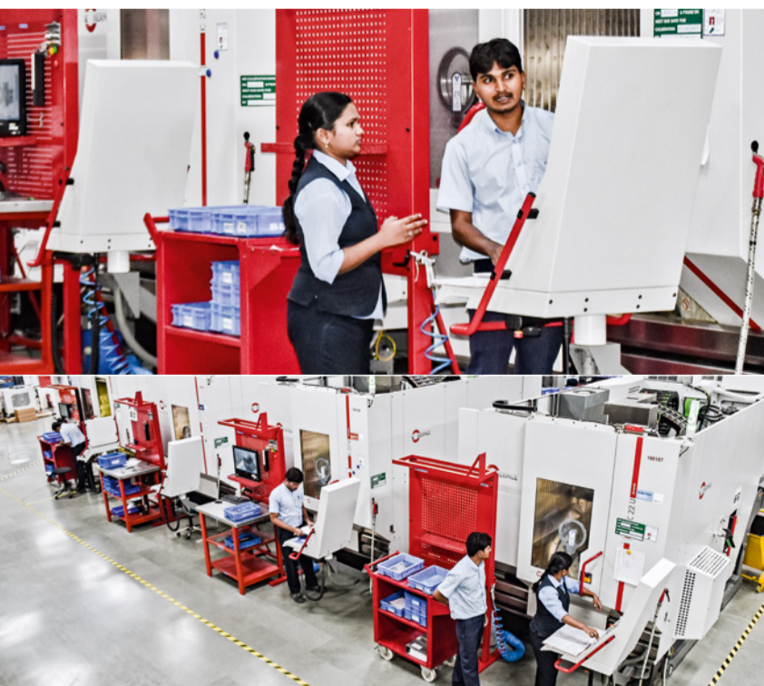
Above Female machine operators are also employed; SECO Tools India is playing a leading role in their employment across the country. below Several 5-axis machining centres C 22 U in tool production.
