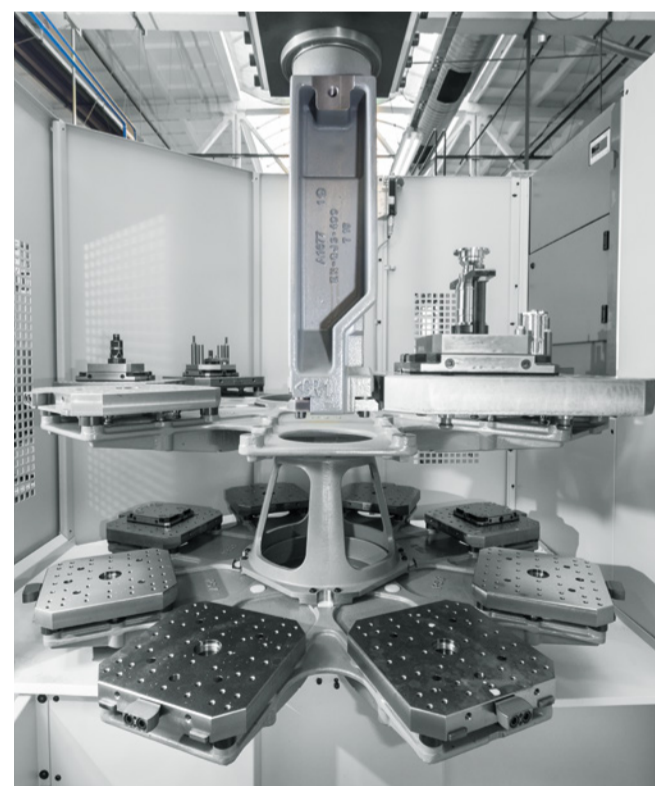
Pallet changer PW 150 of the C 22 UP machining centre featuring a total of 18 pallet pockets in the complete system, configured for pallet size 320 x 320 mm with max. pallet weights up to 2 x 150 kg
