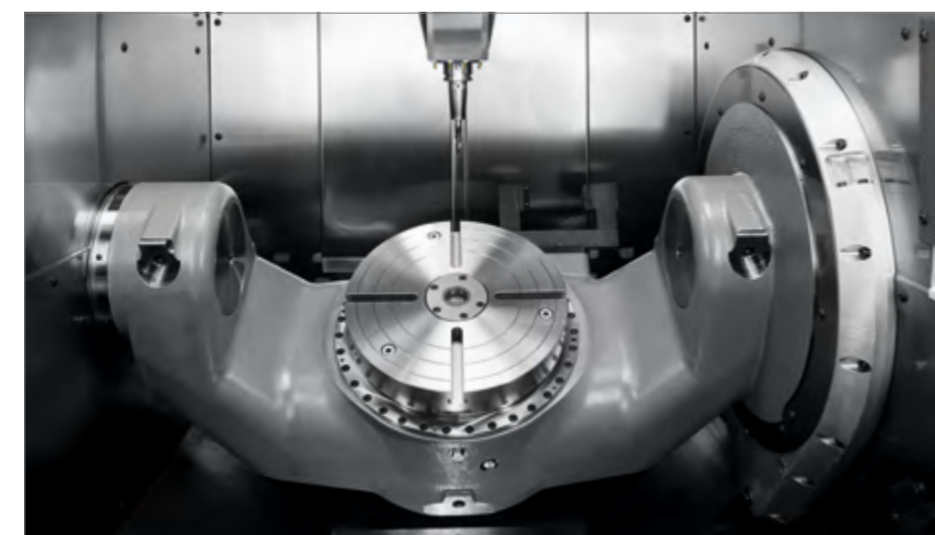
The „Torque“ NC-swiveling rotary table – ideal for 5-axis technology.
