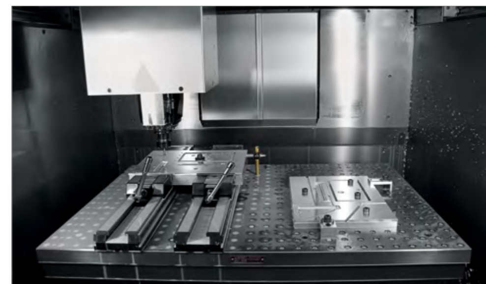
Large working area of the C 40 V machining center with X = 850 mm, Y = 700 mm and Z = 500 mm and the rigid clamping table with clamping surface 1070 x 700 mm. The table is designed for universal applications with standard and special clamping devices. The slim design of the Z axis or milling spindle provides excellent accessibility for 5-sided surface machining.
