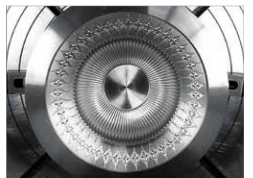
Filigree milled molding die of a shell with fine detailing.
