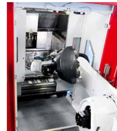
Left: Robot handling a pallet. The robot retrieves the pallet with the finished part and places it in the magazine, then picks a pallet from the rack and places it on the predetermined machine table. The robot is also responsible for pallet handling from and to the setup station.
