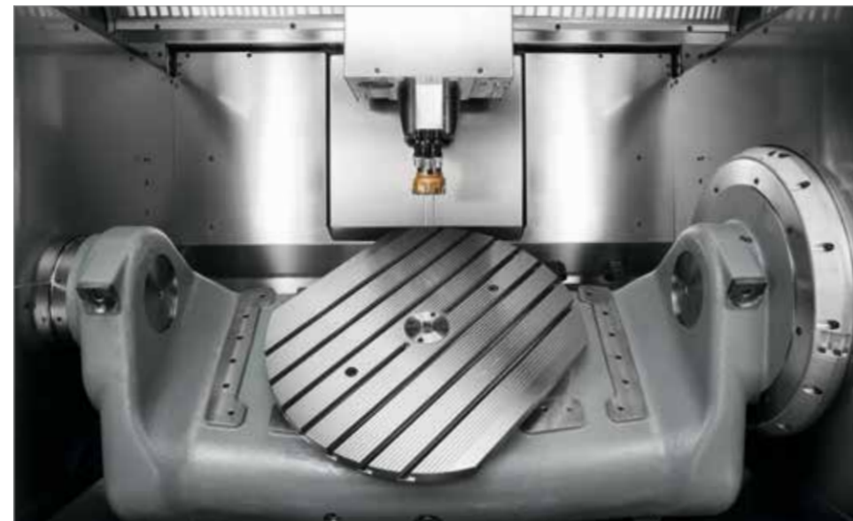
Various NC swivelling rotary tables provide the ideal entry into 5-axis technology.
