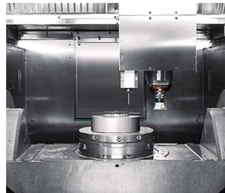
Working area of 5-axis machining center with integrated MPA technology, manufacturing a tool insert.
