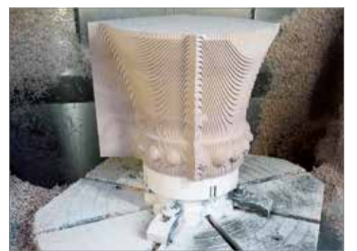
Working area of the Hermle-MC C 30 U with NC swivelling rotary table (Ø 630 mm) for 5-axis complete machining of demanding prototypes, models and tool segments in 3D form.
