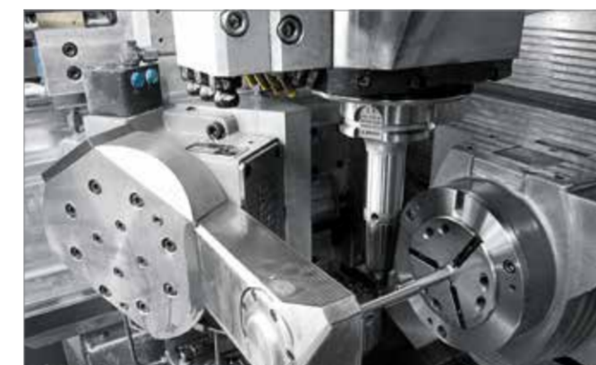
Machining a long cantilevered special tools holder on the Hermle C 40 U machining center with arbor holder; the arbor holder is seated on a slide and permits machining of up to 250 mm long parts as well as corrugated parts.
