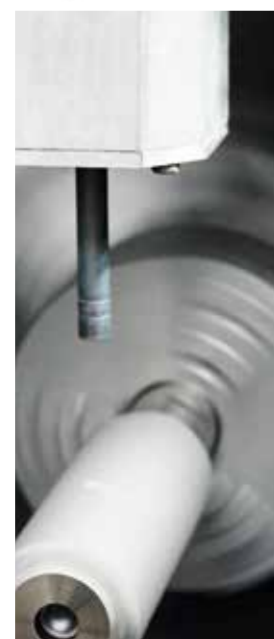
Manufacturing of a shaft with cooling channel made of 1.2344 (temperable hot-working steel, H13).
