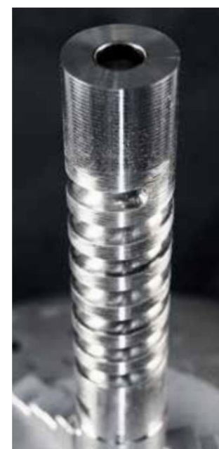
Manufacturing of a shaft with cooling channel made of 1.2344 (temperable hot-working steel, H13).
