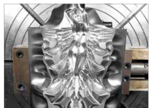
Other molding die made of special cast iron for casting of an exclusive crystal glass sculpture.
