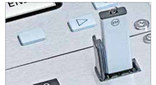
2 Storage media can be connected to the control panel quickly and easily via the USB-2.0 interface.
