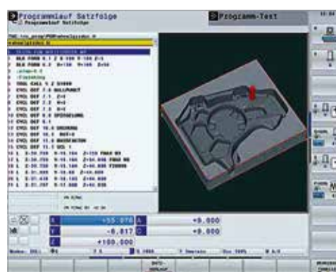
3 User interface: Along with its bright appearance, the display focuses on easy operability for users. Different areas are clearly separated from each other and icons provide information about the different operating modes.
