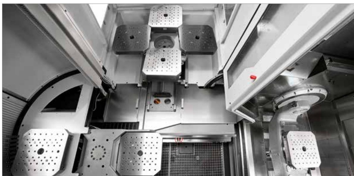
A look at the pallet changer PW 250 with setup station (left), 4x storage (rear), the traversing unit (front) and the machine working area (right).
