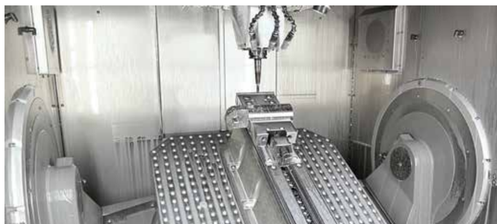
The large working area (1000 x 1100 x 700 mm, X/Y/Z) of the 5-axis machining centre's C 50 UP and the NC rotary table 700 mm in diameter for pallets 800 x 800 mm to hold workpieces weighing up to 2000 kg.
