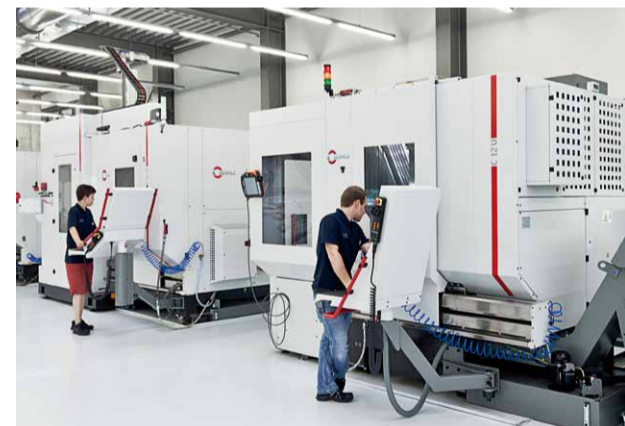
Left: The working area of the five-axis C 22 U machining centre with the swivelling rotary table on which a multiple clamping system is installed. Right: The line of five-axis machining centres: the C 22 U featuring PW 150, the C 12 U with RS 05, and the C 40 U in the new production centre at Fetzer Medical GmbH & Co. KG
