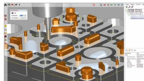
MPA Studio calculates and simulates application paths as well as machining paths for the MPA process.
