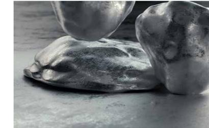
A binding contact surface is created between the powder particle and the substrate.
