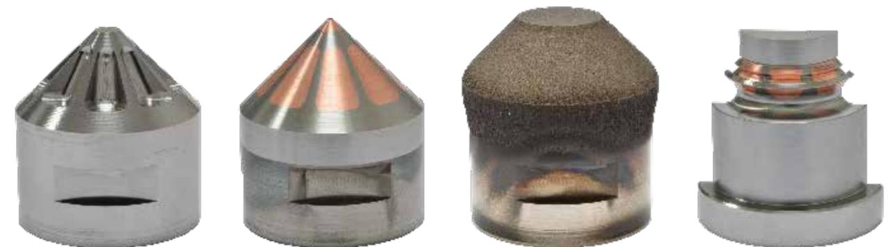
Manufacturing stages of a tool with copper cores. In a steel blank, pockets are defined and then filled with copper via MPA. After milling the cone surface, a steel cover is applied. Ultimately, the final component contours are milled.
