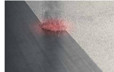
When impacting with the substrate, the metal particles carry a vast amount of kinetic energy which is converted into plastic deformation of the material.
