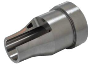
Sprue bush for plastic injection moulding. The embedded copper conducts the resulting heat to the cooling channel.
