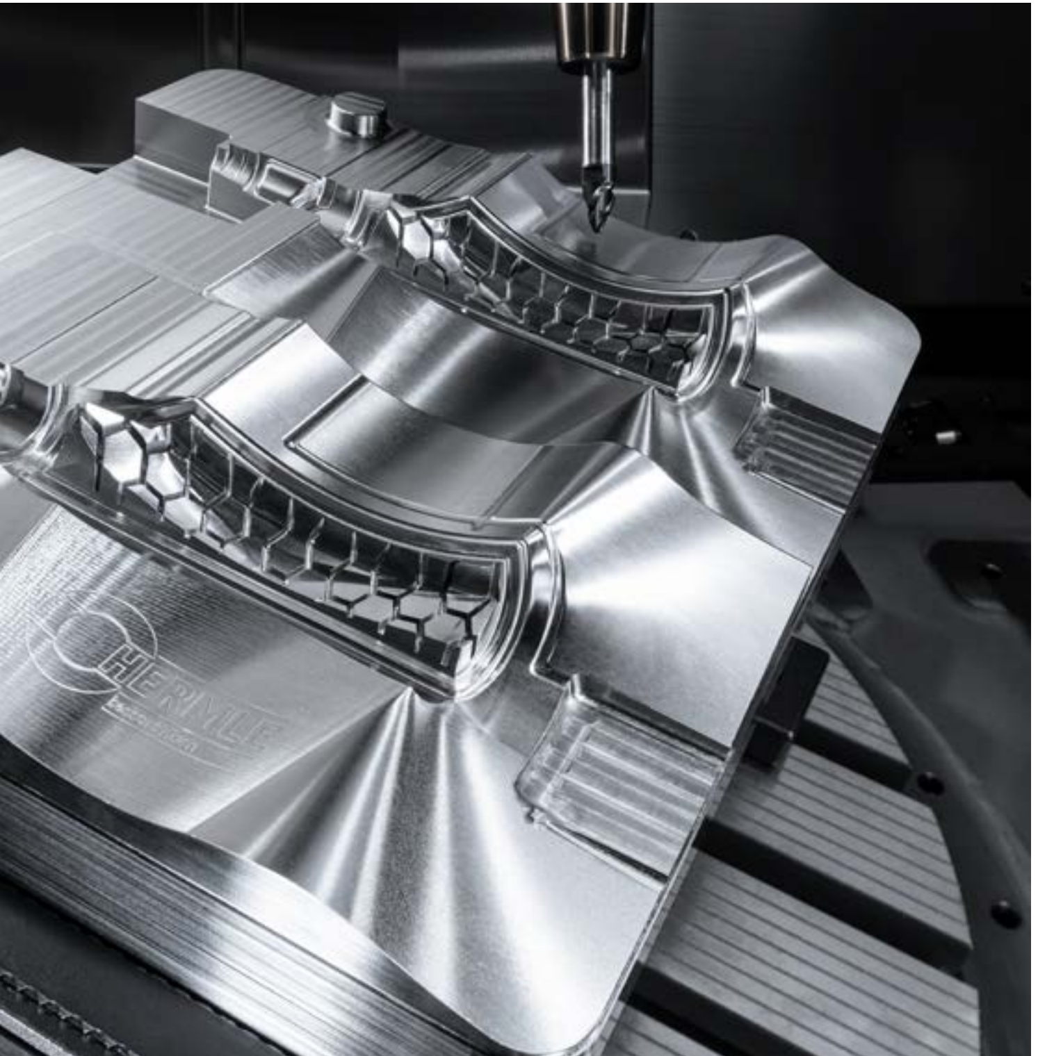
HERMLE C 42 U dynamic in 5-axis version | Machining of a die for toolmaking and mould construction.
