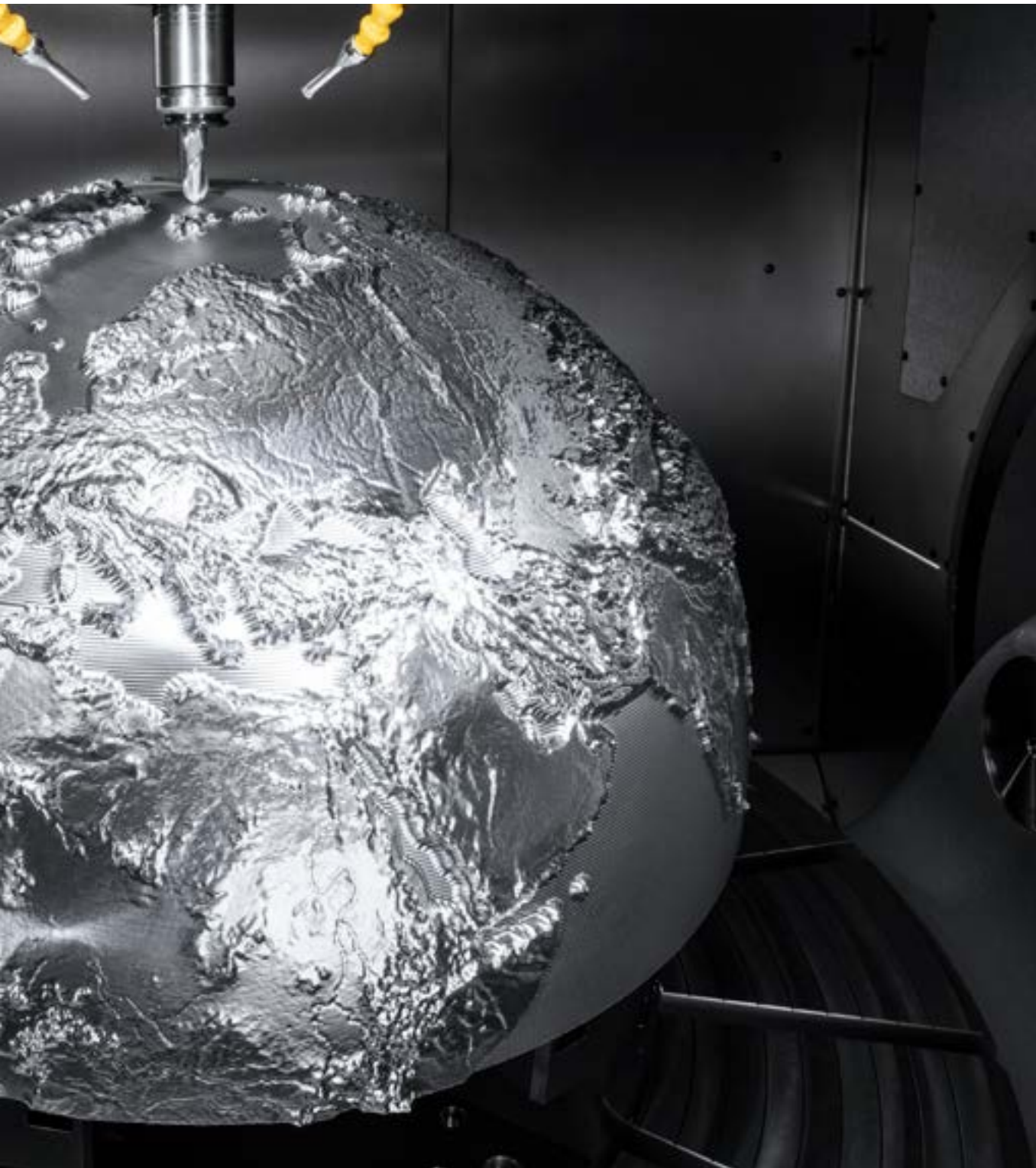
HERMLE C 62 U MT dynamic in 5-axis mill-turn version | Machining of a globe for model making.
