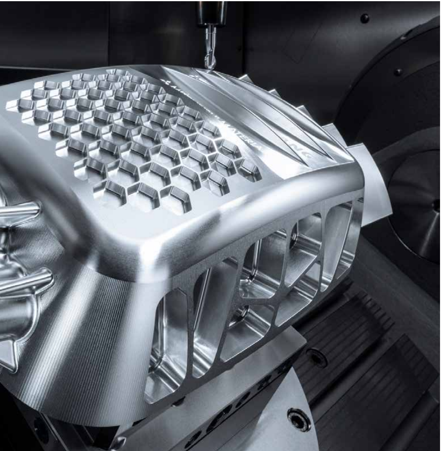
HERMLE C 42 in 5-axis version | Machining of a technology component for the aerospace industry.
