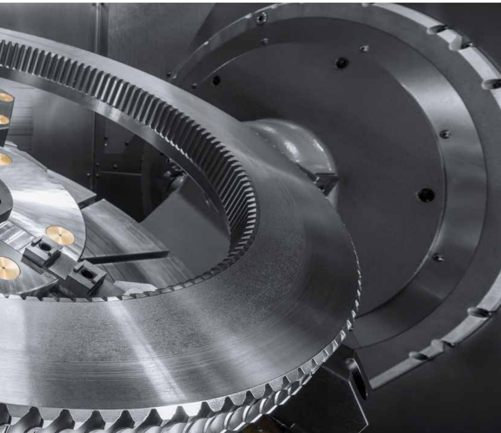
Machine construction. Gearwheel with worm gear external splines and straight internal splines produced by hob peeling.
