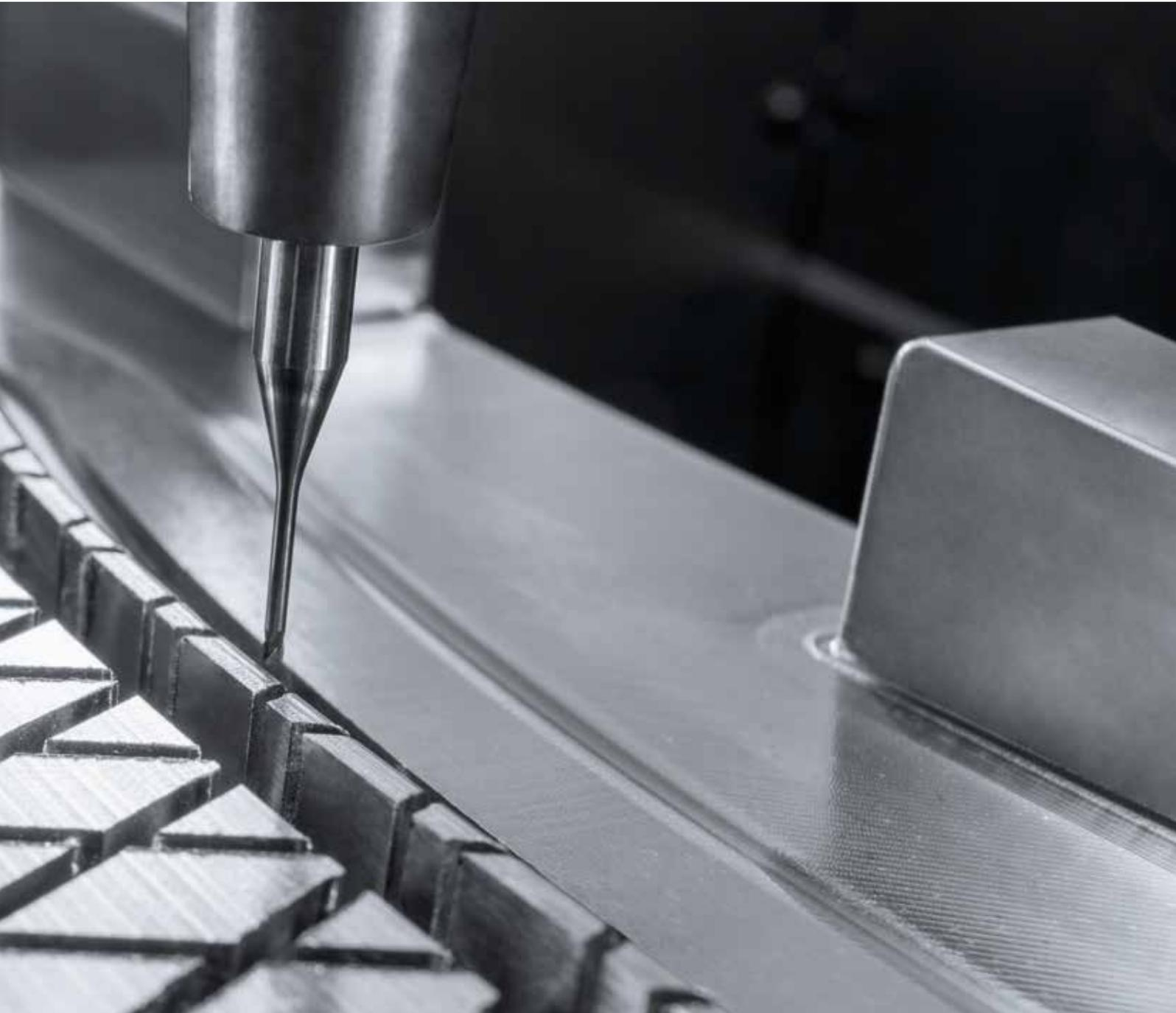
Tool and mold making. Rib component made of tool steel for a shoe sole die mold.
